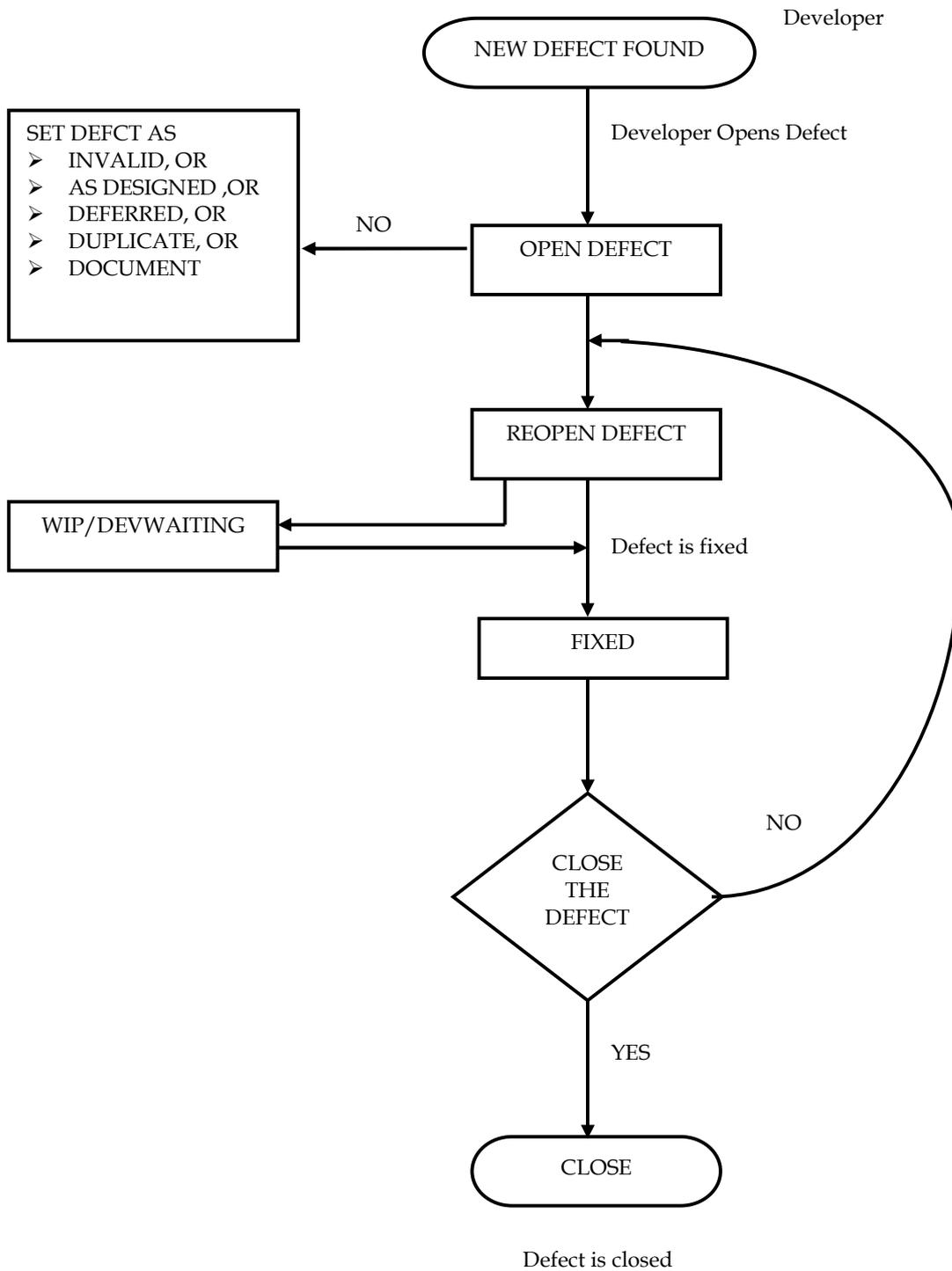
Fig. 2. Represent Defect Life Cycle
